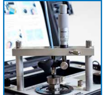
PROXIMITY OPTION 9100-PPA01 fixture is used to check the static and dynamic output of an eddy current proximity probe.
