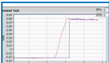
Step Pressure Rise – Transient
